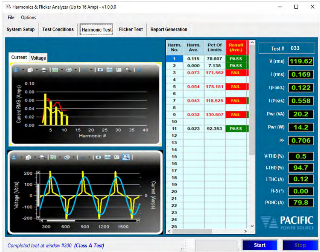
Figure 6-27: Lighting product < 25 Watt that fails all 3 tests per Clause 7 of IEC 61000-3-2 (2018)
