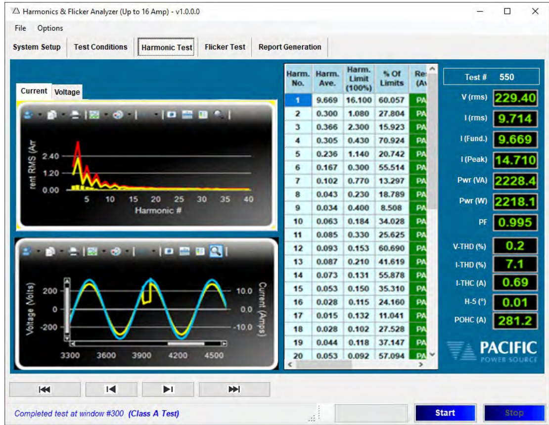
Figure 6-24: Short Glitch during Harmonics Test revealed during Replay
