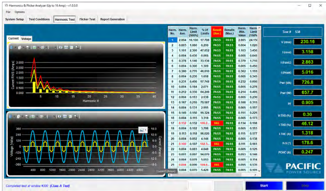
Figure 6-6: Harmonics Test Class A FAIL display, "stretched" to include all data column
