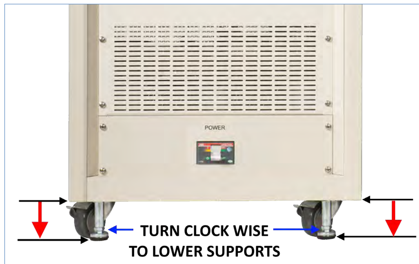
Figure 5-2: Lower All Four Cabinet Corner Supports to Support Cabinet weight
