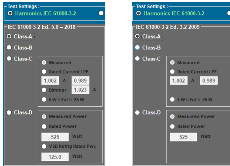
Figure 6-30: Test Settings for IEC 61000-3-2, Ed. 3.2 versus Ed 5.0
